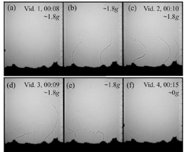
*Photographs of the evolving mushy-layer system featuring freshwater plumes in various gravities: Panel (a) shows freshwater plumes beginning to rise from chimneys shortly after the onset of hypergravity. Panels (b) and (c) illustrate the coupled oscillatory behavior of the plumes in hypergravity. Panels (d) and (e) provide a clear view of the Rayleigh-Taylor instabilities in horizontal jets observed in hypergravity. Panel (f) features inertial plumes shortly after the onset of microgravity.*
