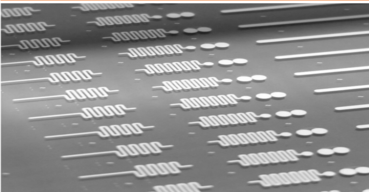
Array of transmons and resonators by Chris Axline, Ph. D., from Schoelkopf Group
